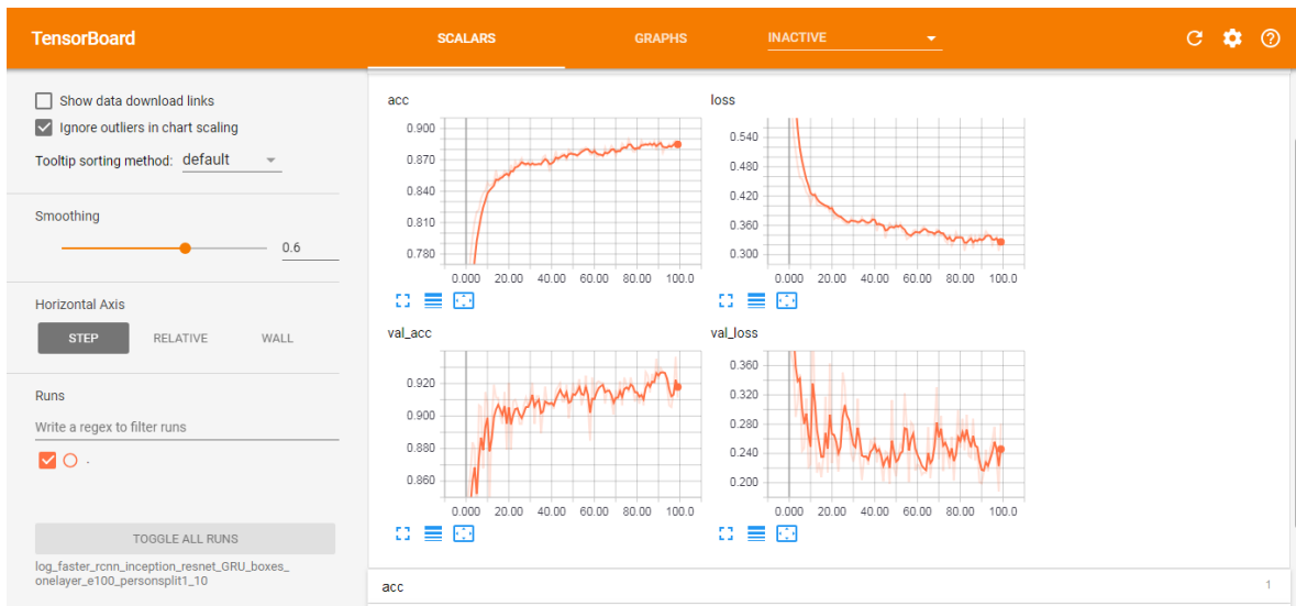
Figure 6.2: The interface of TensorBoard displaying the training loss (upper right graph), training accuracy (upper left), testing loss (bottom right) and testing accuracy (bottom left).
