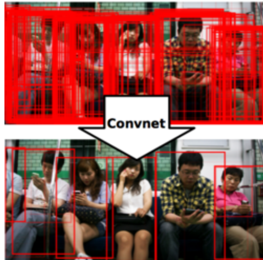
Figure 2.8: Example of non-maximum suppression using a convnet [37].
